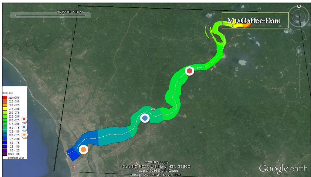
Figure 5-6 Flood inundation map on day 4 at 5:30am (i.e. 16hr 22 min. after breach)
